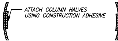
SHIP LAP JOINT (TYPICAL FOR STRUCTURAL COLUMNS)
